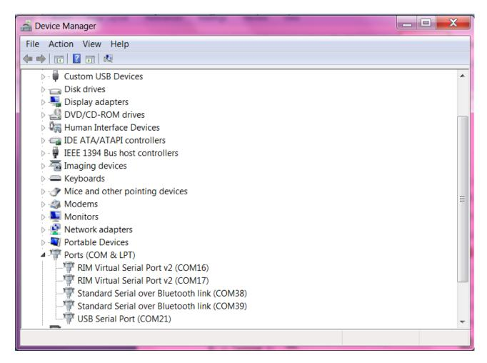
COM21 above shows the USB Serial port device.
