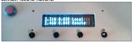
Power consumption and battery resistance is shown when button 4 is pressed twice.
