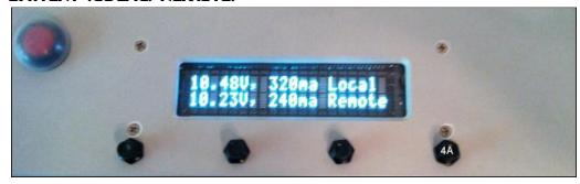
Local and remote battery voltage and current consumption is shown when button 4 is pressed once.
