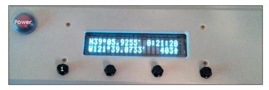
Power on the unit, by default position is shown. Pressing button (1) will show position in Decimal degrees. When 3D lock is established, the altitude is shown (in Feet) and alternates between an airplane icon and Ft symbol. When 3D lock is lost, the characters "------ are shown.
