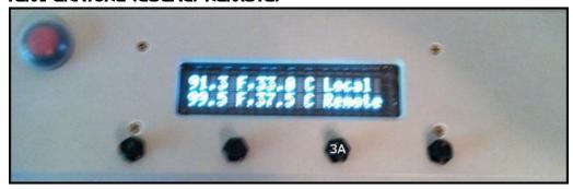
Local and remote temperature is displayed in Fahrenheit and Celcius when button 3 is pressed once.
