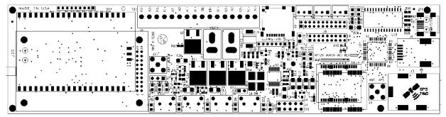
Assembled height: ½" High (fits inside 54mm Performance Rocketry AF Tube, slip fit in Coupler)
