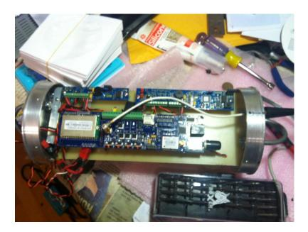
Use a ¼-20 drill bit for the RPSMA antenna socket. Drill the hole and put the nut on the top, screw in antenna. Optimally, the GPS shall be pointed up and the RPSMA pointed down or out of the way of the GPS antenna. External GPS antenna if needed.
