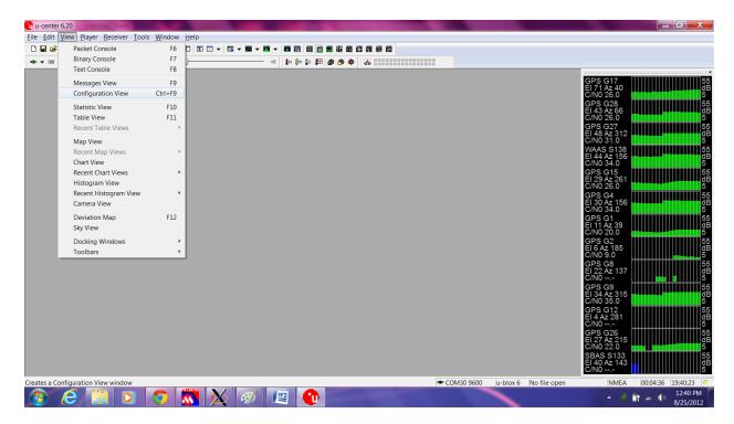
6. Verify that the configuration data will be saved to the device (BBR, FLASH, I2C EEPROM selected)
