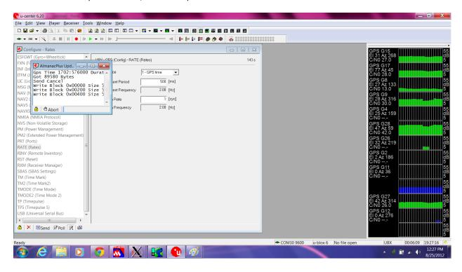
The unit is now configured. Be sure to leave the GPS Battery connected to the module so that the GPS Almanac data is preserved up to and during flight. Should the GPS lose telemetry lock during flight, the GPS battery will ensure hot-start and re-acquisition of fix in < 1 second with hot-start enabled.
