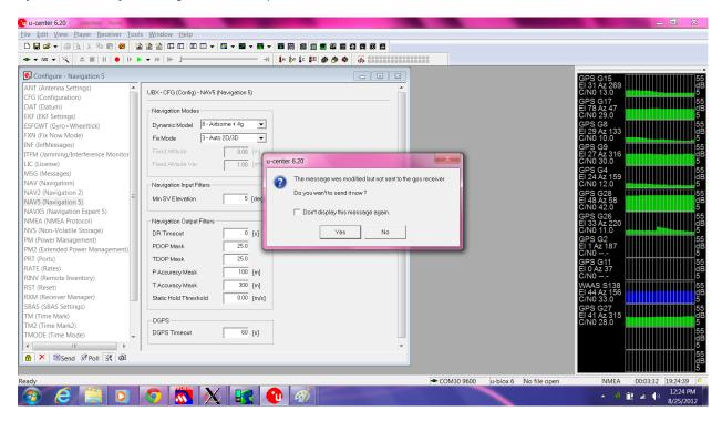
8. Verify the Rate is set to 2HZ (500msec) for 1-second real-time response with the Base station receiver
