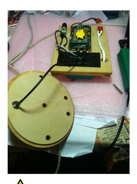
Always verify that the RPSMA connectors are tightened both on the board and antenna using a 5/16" nutdriver or 5/16" wrench. Do NOT tighten too hard, only confirm they are cranked and attached completely. Do NOT yank on the RPSMA cables.
