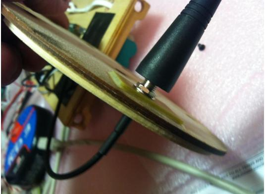
Verify that when tightened, the antenna is seated. Having clearance confirms the fit.
