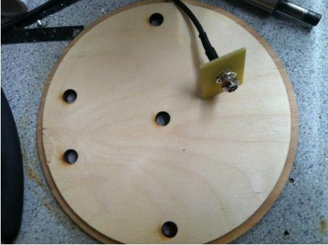
A 1/8" piece of G10 cut into a 2x2 or 2x1 rectangle with a ¼" hole drilled in the middle is glued on top of the bulkplate. A hole which is ½" in diameter is drilled away from all metal parts for the RPSMA to fit through. The Polecat Aerospace components are laser-cut, ensuring proper sled alignment and no bind of all-threads.
