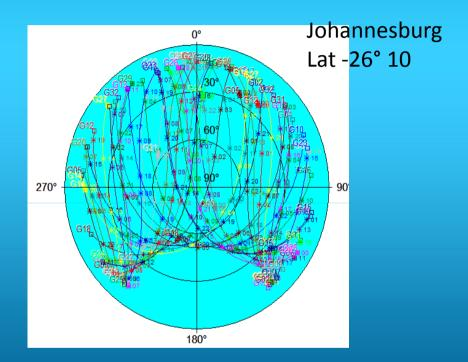
Even though the area of the sky where satellites can be seen are almost identical, Taipei has a gap to the North and Johannesburg has a gap to the South, the graphs on page 15 show very different results. This difference highlights the need for longer data logs.
