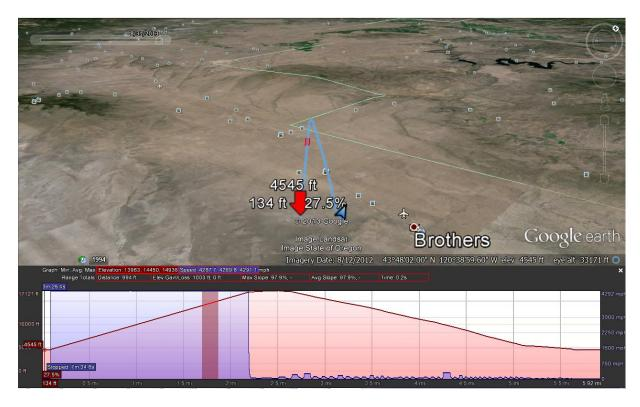
Showing Elevation profile, to the left of the graph, several positions have been provide with an initial altitude of 4545ft. You can use successive measurements or an average. In the example above, successive measurements determine that the launch site is 4,545 MSL; ground level is 4,545 MSL.
