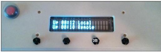
System uptime in HH:MM format is displayed when button 3 is pressed a second time.
