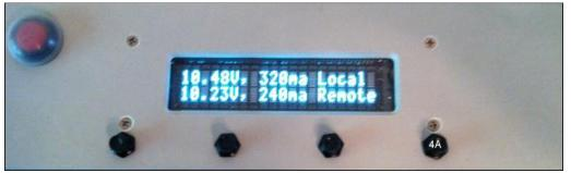
Local and remote battery voltage and current consumption is shown when button 4 is pressed once.
