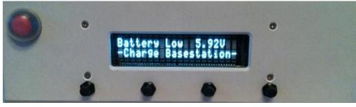
When battery voltage drops to 6V and below, the base-station needs to be charged.
