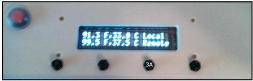
Local and remote temperature is displayed in Fahrenheit and Celcius when button 3 is pressed once.
