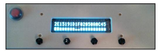
Pressing button (2) displays the Satellites available to the remote receiver as well as their relative signal strength (using a 2 column bar-graph to depict a 1-10 value). Two digits are used for each Satellite and the SVN is shown in hexadecimal above the signal strength indication (to constrain SVN numbers to 2 columns). Currently active US satellites are listed below:
