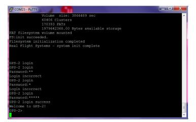
Reboot the Base-Station. When the Base-station boots, you will see a message on the console asking for input, ignore it (do not hit enter).
